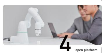
The integrated controller is open, and COBOTTA's control API is made public, allowing creators to develop their own applications in the environment they choose (OSS version).
