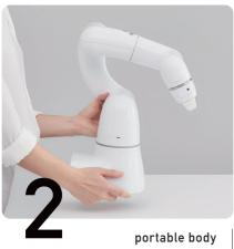
The main unit weighs approximately 4 kg providing easy portability, and offers a load capacity of 500 g. The integrated controller not only reduces wiring, but also allows consolidated control with other devices. ORIN is supported as standard.
